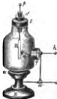
Fig. 13. Gold Leaf Electroscope.
